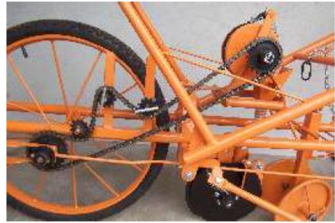
The picture shows how the roller chain is mounted to drive the rotor distribution system.
