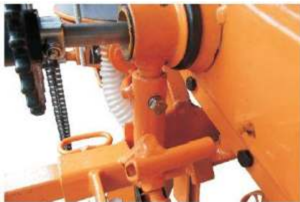
Tighten the armored unit bearing housing in the tubes
