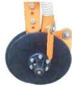
Double disc furrow opener with offset discs
