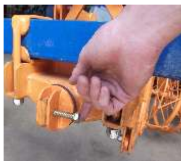
4. Travar com parafuso \frac{1}{2} x 1 \frac{3}{4}
